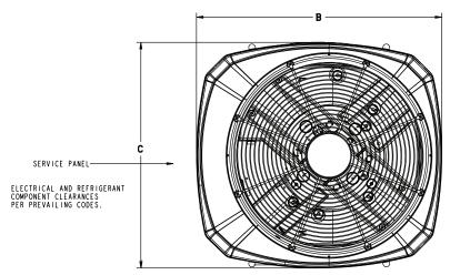
TOP DISCHARGE AREA SHOULD BE UNRESTRICTED FOR AT LEAST 1524 (5 FEET) ABOVE UNIT. UNIT SHOULD BE PLACED SO ROOF RUN-OFF WATER DOES NOT POUR DIRECTLY ON UNIT, AND SHOULD BE AT LEAST 305 (12") FROM WALL AND ALL SURROUNDING SHUBBERY ON TWO SIDES. OTHER TWO SIDES UNRESTRICTED.
