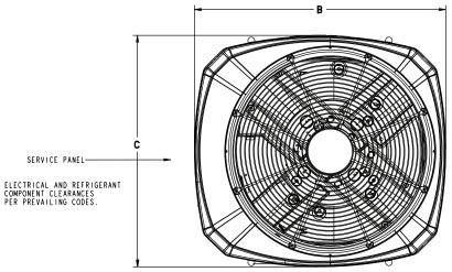
TOP DISCHARGE AREA SHOULD BE UNRESTRICTED FOR AT LEAST 1524 (5 FEET) ABOVE UNIT. UNIT SHOULD BE PLACED SO ROOF RUN-OFF WATER DDES NOT POUR DIRECTLY ON UNIT, AND SHOULD BE AT LEAST 305 (12") FROM WALL AND ALL SURROUNDING SHUBBERTY ON TWO SIDES. OTHER TWO SIDES UNRESTRICTED.
