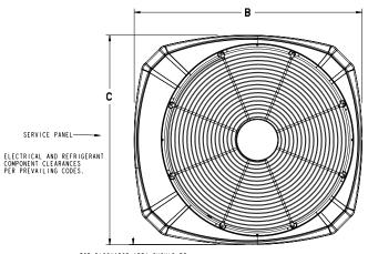
TOP DISCHARGE AREA SHOULD BE UNRESTRICTED FOR AT LEAST 1524 (5 FEET) ABOVE UNIT. UNIT SHOULD BE PLACED SO ROOF RUN-OFF WATER DOES NOT POUR DIRECTLY ON UNIT, AND SHOULD BE AT LEAST 305 (12") FROM WALL AND ALL SURROUNDING SHUMBBERY ON TWO SIDES. OTHER TWO SIDES UNRESTRICTED.
