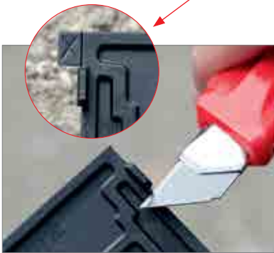
1. Remove Area X and Clip B on the left and right with the cutter
