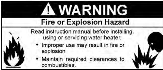
Minimum clearances between the water heater and combustible construction are 0 inch at the sides and rear, 5.5" (14.0 cm) from the front and 18" (45.7 cm) from the top. (Standard clearance.) If clearances stated on the heater differ from standard clearances, install water heater according to clearances stated on the heater.
