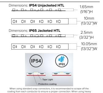
duty snap connectors, this is only necessary for IP65 and IP68 types.
