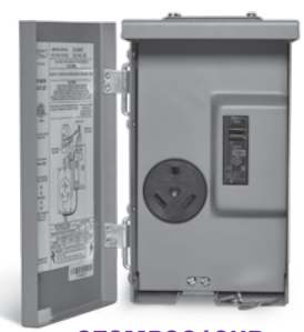
CESMPSC13HR TT-30 travel trailer receptacle Breaker: 1P 30A
