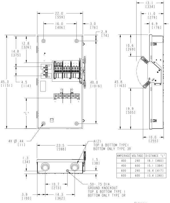
Dimensions shown in inches and millimeters [ ]. Dimensions shown accurate to  $\pm$  1/8 inch.
