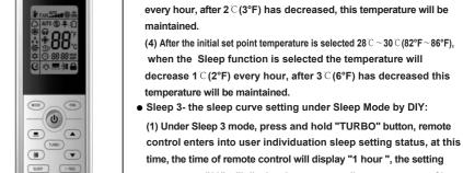
(2) Adjust ▲ and ▼ button, could change the corresponding setting temperature, after adjusted, press "TURBO "button for
