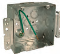
"H" Bracket Narrow bracket allows side-by-side mounting on stud. Positioning tabs locate box perfect distance from stud. V notch centers box. Dimples protect flush drywall installation.
