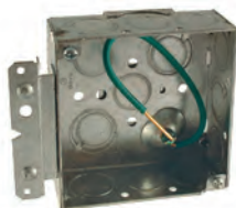
"H" Bracket Narrow bracket allows side-by-side mounting on stud. Positioning tabs locate box perfect distance from stud. V notch centers box. Dimples protect flush drywall installation.
