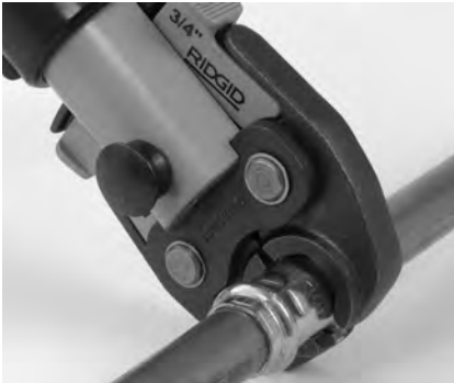
Figure 7 – Placing Scissor-Style Jaws Around Fitting
