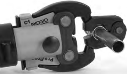
Figure 10 – Attaching Actuator to Press Ring
