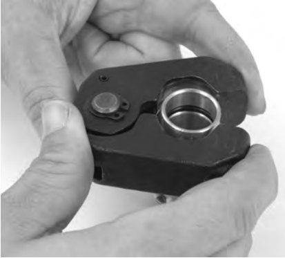
Figure 9 – Installing Press Ring onto Fitting
