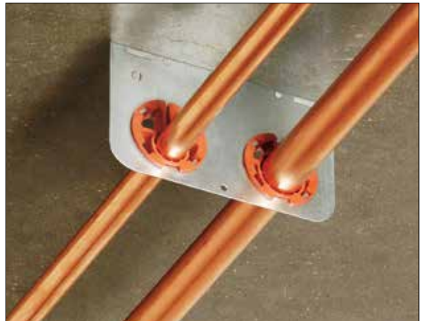
PipeEye Suspension brackets are designed with the same 1-11/32" hole as a standard metal stud punch for use with PipeEye grommets. Secure the brackets directly to ceilings, decks, walls or vent pipes for tight installations where space is limited.
