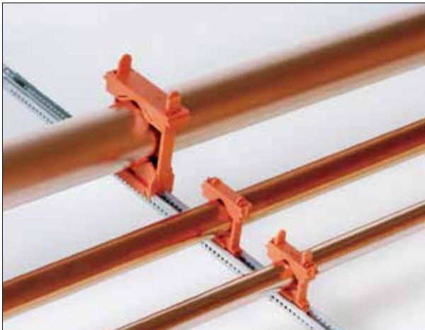
E84 TouchDown clamps and TouchDown II clamps fit PowerBar and PowerBar Mini Strut brackets. The releasable locking mechanism allows for variable clamping tension for expansion and contraction. Clamping ranges are 1/2" - 2" CTS or 3/8" - 2" IPS (Schedule 40).
