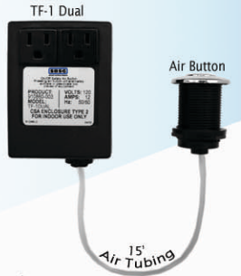
▲ Shown: Actual connection configuration. Air button is mounted in sink or surface of choice. 1 3/8" diameter hole required.
