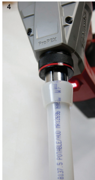
Expansion with Milwaukee M18 ProPEX expansion tools
