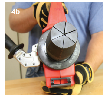
Correct expansion head alignment
