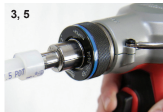
Expansion with Milwaukee M12 ProPEX expansion tools
