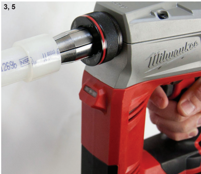
Expansion with Milwaukee M18 ProPEX expansion tools
