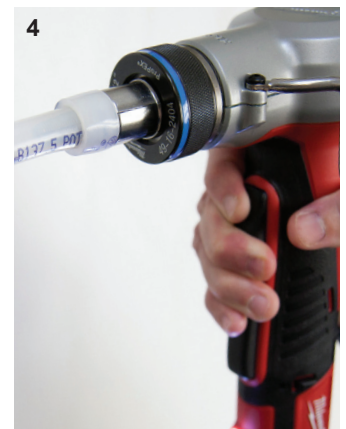
Expansion with Milwaukee M12 ProPEX expansion tools
