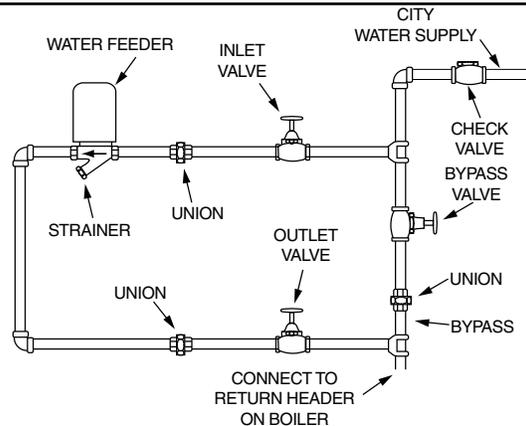
2. Water feeders are shipped from the factory equipped for a 2 gpm feed rate. A separate kit with instruction sheet and field installable orifices for 1 gpm and 4 gpm feed rates is included. If the alternate feed rates are required, refer to the instruction sheet provided with the kit for orifice replacement.
